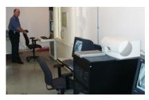
A multiple work station consists of the main X-ray system and, on the right, networked computers for the remote inspection of images. Source: X-Ray Associates LLC
