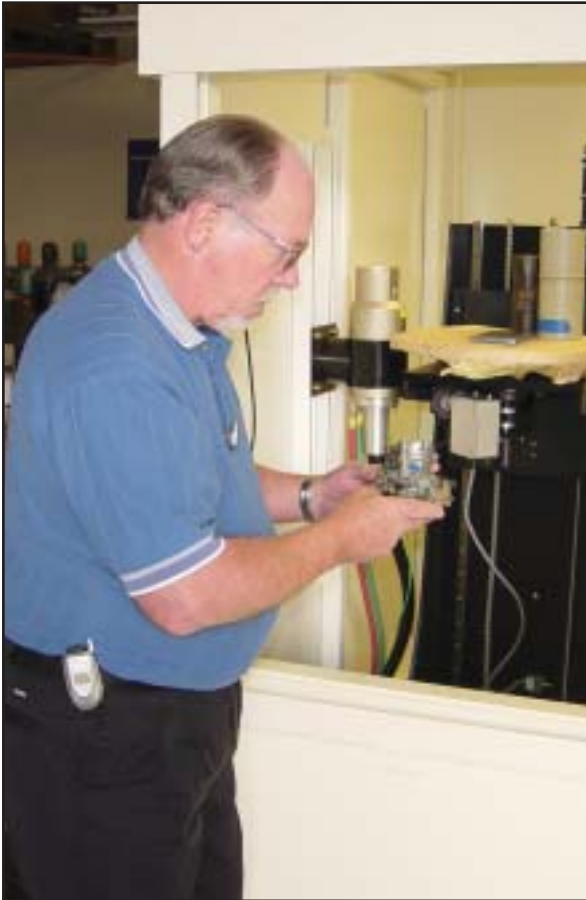
A sample is loaded onto the 5-axis manipulator. It puts the part between the X-ray source and the image-capture device. Photo: David Pugsley
