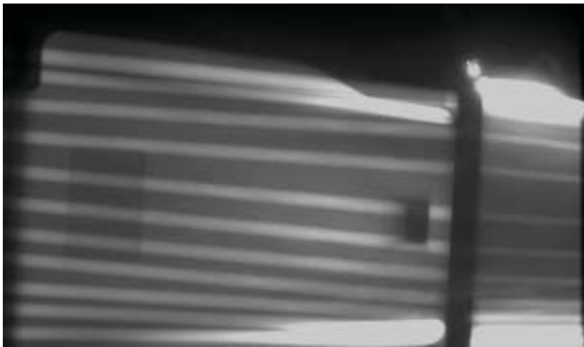
The real-time digital X-ray technology can inspect both the length of the blade, as seen here, and the hole intersections at the same time. Film would require two or more exposures. Photo: David Pugsley
