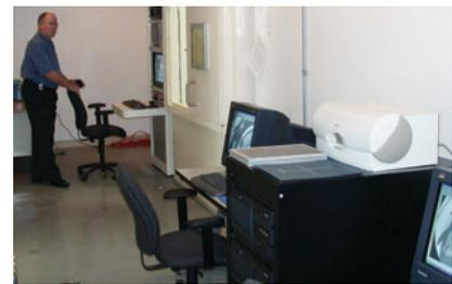
**A multiple work station consists of the main X-ray system and, on the right, networked computers for the remote inspection of images. Source: X-Ray Associates LLC**
