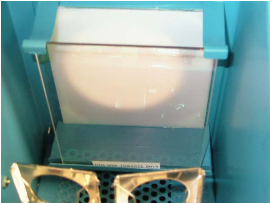
HEAT GLASS INSTALLED WITH STICKER "THIS SIDE TOWARDS BULB"
